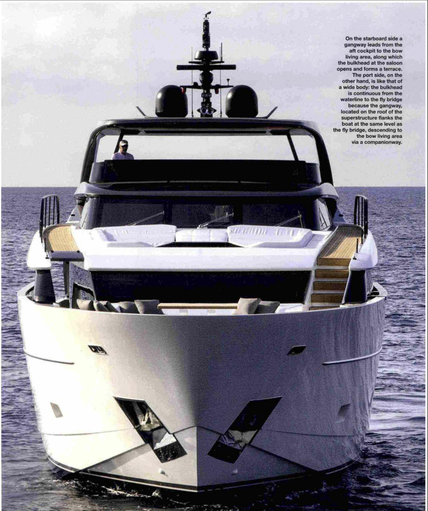
On the starboard side a gangway leads from the aft cockpit to the bow living area, along which the bulkhead at the saloon opens and forms a terrace. The port side, on the other hand, is like that of a wide body: the bulkhead is continuous from the waterline to the fly bridge because the gangway, located on the roof of the superstructure flanks the boat at the same level as the fly bridge, descending to the bow living area via a companionway.
